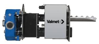
measurements can be significantly reduced with Valmet DS. Also, uniquely to Valmet DS's measurement technology, the sample is extracted from falling cake flow after a centrifuge or screw press, before returning the sample material back to the process. Continuous measurements mean the results can be immediately utilized without needless delay from manual sampling and laboratory analysis. This offers better feedback control and real-time assessment of dewatering efficiency.
