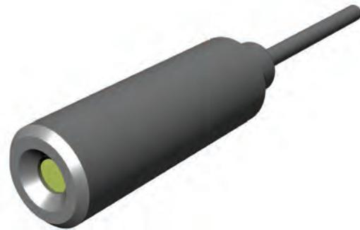
The 420 series of 4-20mA pressure transducers are a cost effective and robust solution designed for continuous water level measurement where a 4-20mA output is required. It may be used with other liquids that are compatible with its wetting materials which are UPVC, Nitrile and Aluminum Oxide. Different choice of seals is available for other applications. The sensor includes temperature and barometric pressure compensation.
