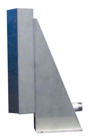
KUH KAI is an innovative product that collides, stirs and breaks down sludge and air into fine particles in a pentagonal cylinder 65cm in length, to accelerate the purification of waste water. Air jetted from a pentagonal cylinder diffuses and radiates outward while eddying in a non-conventional approach.
