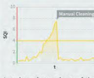
A prolonged exceedance of the SQI threshold value may be an indication for a contamination of the measuring head. In these instances, it is advisable to perform a manual cleaning of the measurement head. If the cleaning resolves the issue the SQI should drop back down to a lower level.
