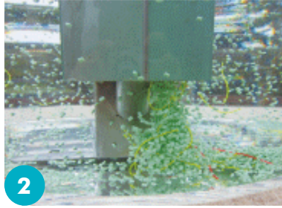
2 Sludge drawn into a cylinder rises and rotates while colliding against and being mixed with air.
