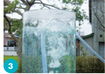
3 Sludge stirred in the cylinder churns in a spiral and circulates in the tank for purification.
