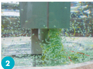
Sludge drawn into a cylinder rises and rotates while colliding against and being mixed with air.
