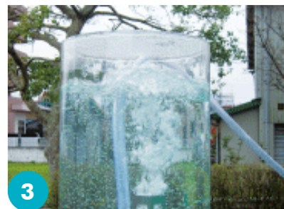
Sludge stirred in the cylinder churns in a spiral and circulates in the tank for purification.
