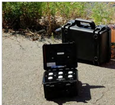
Left: ALERT LAB being used in a water quality analysis laboratory. Middle: The equipment during a field operation, analysing six samples simultaneously. Right: ALERT LAB as used by regulatory agency agent in the field.
